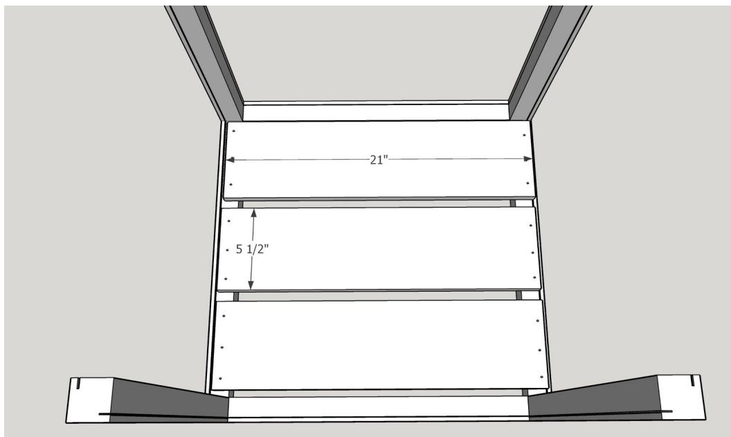
Paint the exterior of the frame, PVC panels and remaining frame pieces. Slide the PVC panels down the grooves in the legs of the planter and fit into the bottom groove. There should be  $1 \frac{1}{8}$ " left at the top of the legs.
