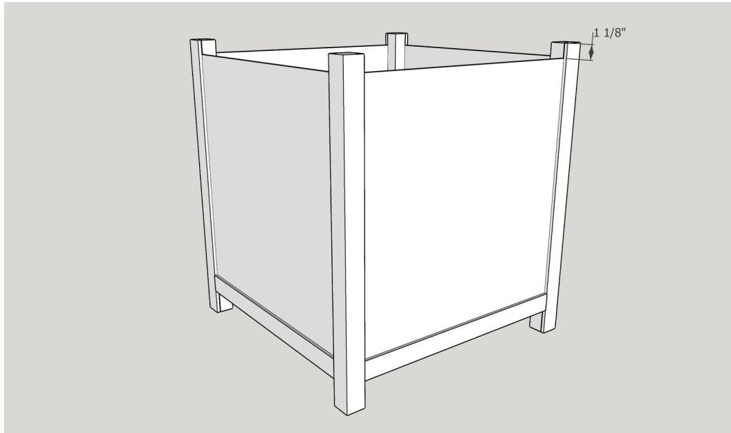
Attach the top 19" pieces with the groove facing down, making sure they are flush with the top of the legs. Screw in place with  $2 \frac{1}{2}$ " pocket hole screws.
