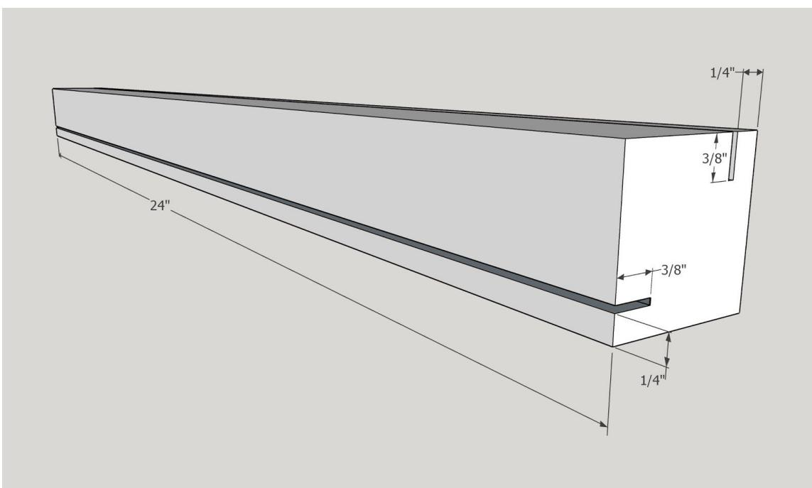
Attach the 19" pieces to the 24" pieces with 2 1/2" pocket hole screws, 2 1/8" from the bottom. All the grooves should be facing up and on the outside edge, lined up with the grooves on the 24" legs.
