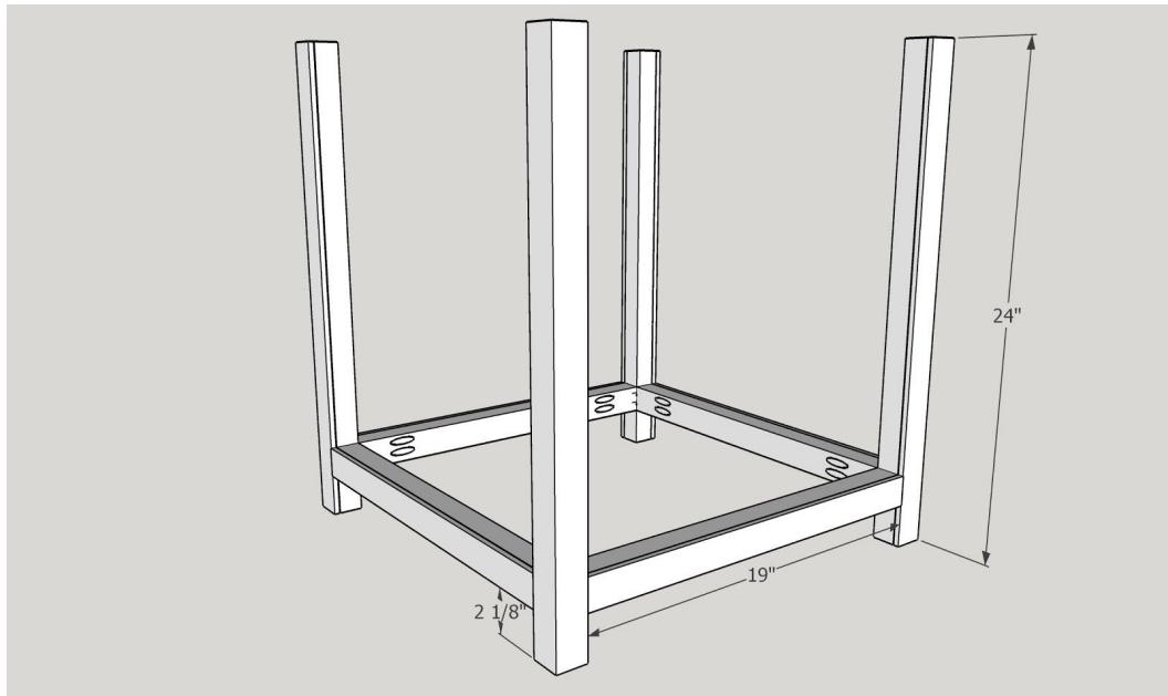
Attach the 21" long cedar fence picket pieces to the bottom of the frame. Allow space in between for water drainage. Make sure the ends aren't covering up the grooves.
