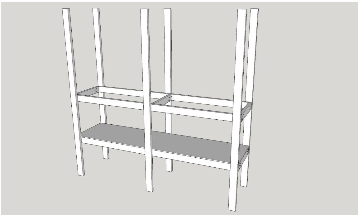
Slide second sheet of 24" x 8' OSB on top and attach around perimeter with 3" screws.
